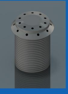
Constructed of extremely corrosion resistant Stainless Steel 316, HeliNozzles operate in conjunction with the HeliSkid Foam deployment system, the HeliNozzle is designed to protect a large area efficiently with either a Foam-Water Mixture or Water alone. The HeliNozzles rapidly suppress fires making the helipad safe for emergency services to complete their rescue efforts.
